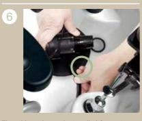
The rubber tube on the installed fixture is now connected to the motor's water outlet.
