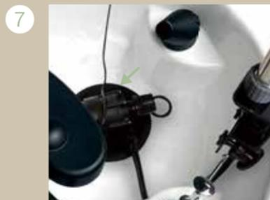
7 Position the motor on the drainage hole of the shampoo bed.
