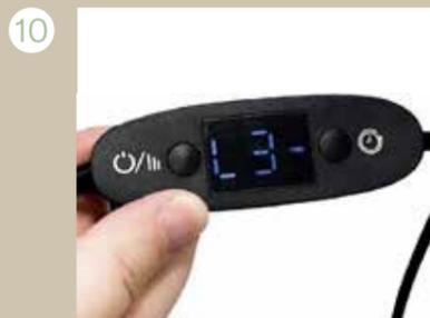
10 Connect the switch and adapter, then press the power button to operate the device. Recommended water pressure level: L3
