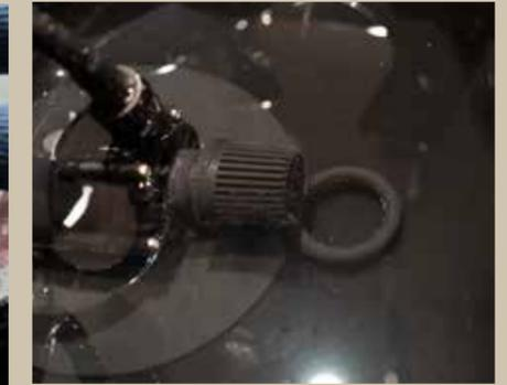
Ensure that the water completely covers the pump in the recirculation system for proper operation.
