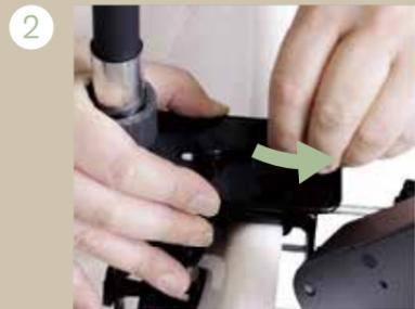
2 The position can be adjusted by moving it left or right before securely tightening the screws. After adjusting the position, tighten the upper screws of the support.
